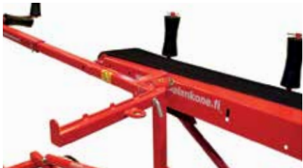
The support is integrated inside the arm.
