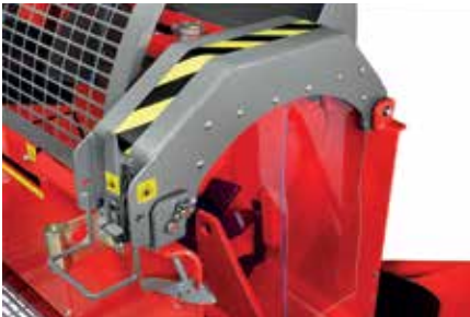
The upper support equipped with a quick-locking mechanism makes the machine structure significantly stronger.
