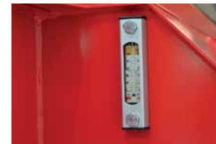
Large oil tank capacity and sight glass.
