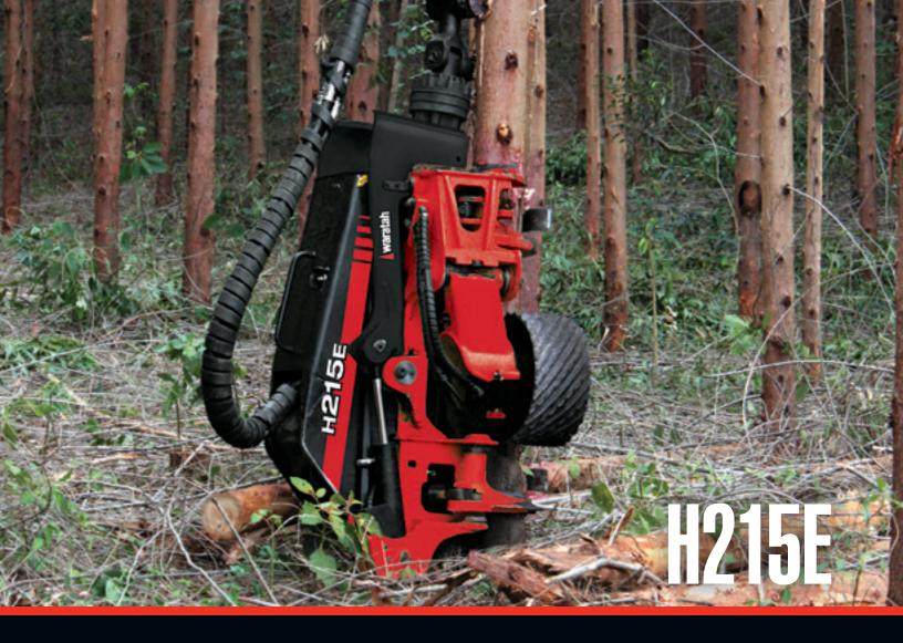
Eucalyptus is no match for the purpose-built H215E. Specifically designed for debarking, this powerful, high-capacity next-generation harvester head productively dominates in the harsh application.
